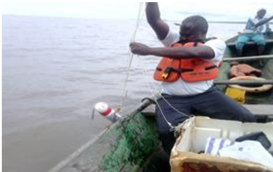
Figure 4. Water sampling with a depth sampler.
